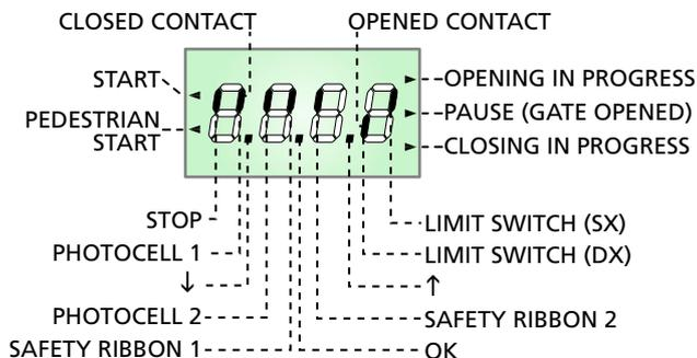
The control panel represents the physical status of the terminal board contacts and of the program mode keys: if the upper vertical segment is on, the contact is closed; if the lower vertical segment is on, the contact is open (the above picture shows an instance where the inputs PHOTO1, PHOTO2, EDGE1, EDGE2 and STOP have all been correctly connected).
